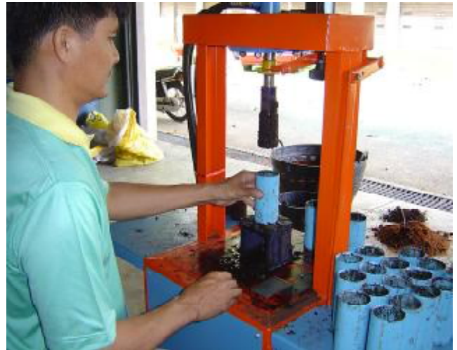
Fig. 1 Nursery block making machine
